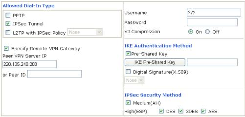
If a *PPP-based* service is selected, you should further specify the remote peer IP Address, Username, Password, and VJ Compression for this Dial-In connection.
