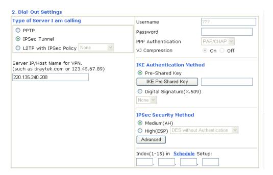
If a *PPP-based* service is selected, you should further specify the remote peer IP Address, Username, Password, PPP Authentication and VJ Compression for this Dial-Out connection.
