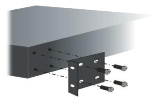
After bracket installation, VigorTalk ATA24 SH chassis could be installed in the rack by using two screws for each side of rack.
