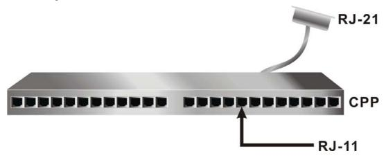
The existing **telephone wiring** usually depends on user's region. Here is the description of typical installation scenario. Use telephone wires with RJ-11 jacks on one end for connecting to the CPP board.
