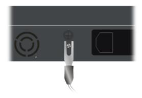
Importance: Please connect the frame ground first before you connect any other cables for this device.
